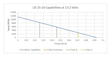
Example of Typical Use Speed-Torque Curve
